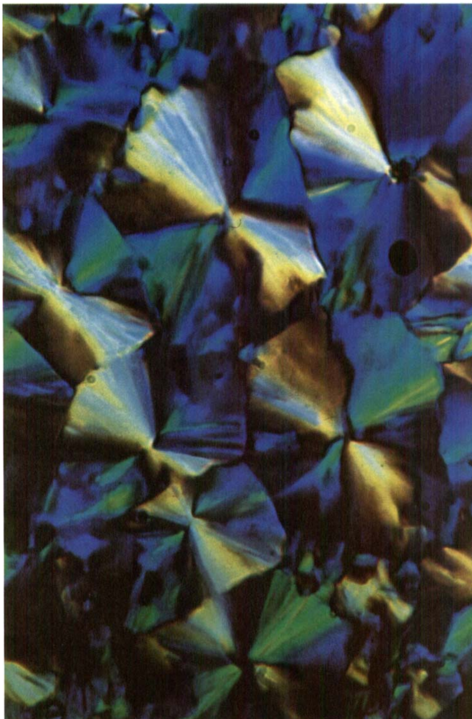
Figure 2. Photomicrograph of 1f in its columnar phase at 60°C viewed between crossed polarizers with an auxiliary wave plate inserted.
